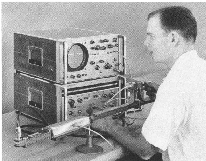
Fig. 1. Waveguide model of P-I-N Modulator can be used on output line beyond coax-to-waveguide adapters or other reflection-producing fittings, and can modulate microwave power with sine waves, complex waveforms, or pulsed signals with extremely fast response. Modulator absorbs microwave power in accordance with instantaneous bias applied to p-i-n diodes and is used here to level microwave power in waveguide system.
